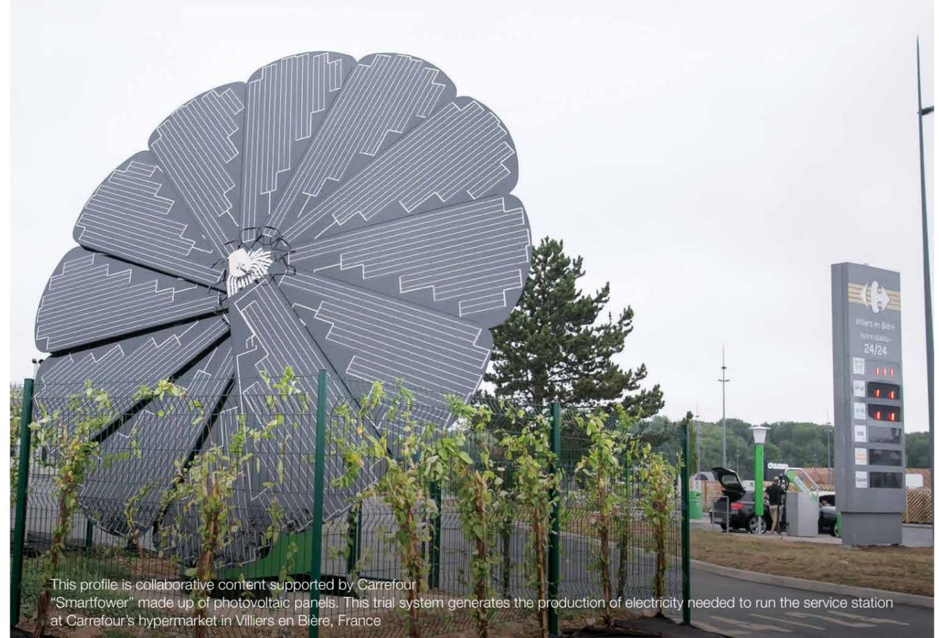
This profile is collaborative content supported by Carrefour "Smartflower" made up of photovoltaic panels. This trial system generates the production of electricity needed to run the service station at Carrefour's hypermarket in Villiers en Bière, France
